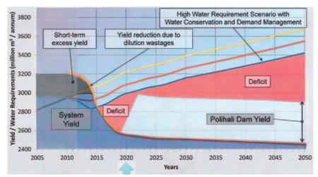
Figure 3: Water balance as it existed in the Vaal River System in 2012
