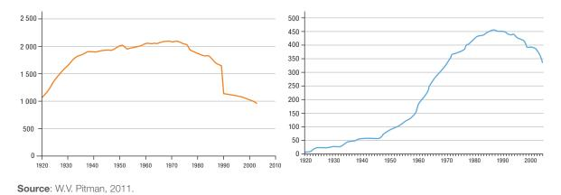
Figure 1: Number and timeline of functioning rainfall gauging stations (left) and streamflow gauging stations (right).
